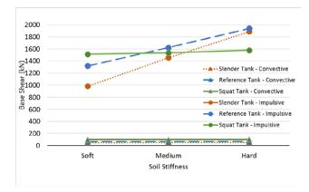
Figure 11. Impulsive and Convective Base Shear vs. Soil Stiffness
