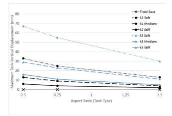
Figure 9. Maximum Tank Dynamic Vertical Displacement vs. Tank Type
