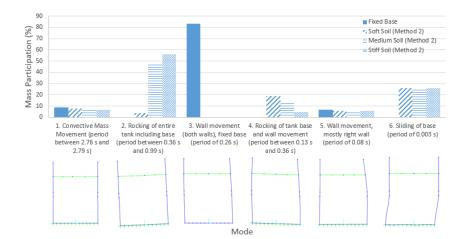
Figure 6. Typical Impulsive Modal Results of the Parametric Study for the Reference Tank
