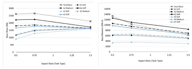
Figure 7. Base Shear vs. Tank Type
