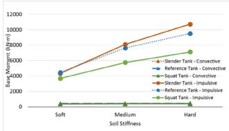
Figure 12. Impulsive and Convective Base Moment vs. Soil Stiffness
