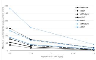
Figure 10. Maximum Wall Horizontal Displacement vs. Tank Type.
